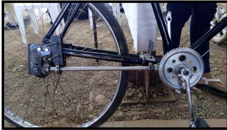
*Fig.1: Shaft driven bicycle*
